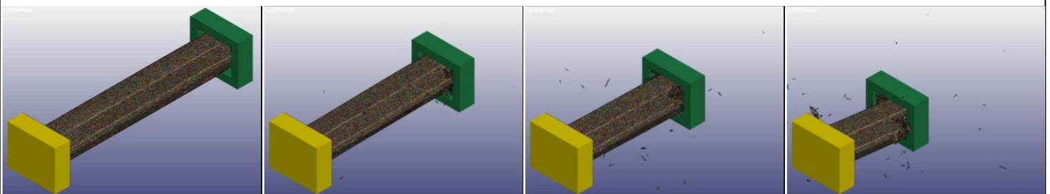
**Explicit Chopped Fiber Crush Tube Simulation**
